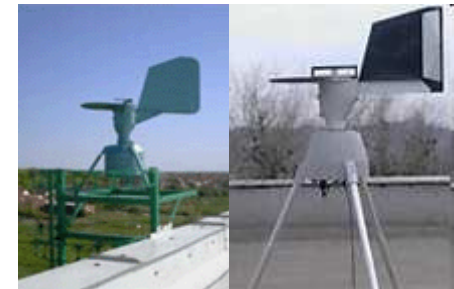
Volumetric pollen and spore trap (Hirst, 1952)
